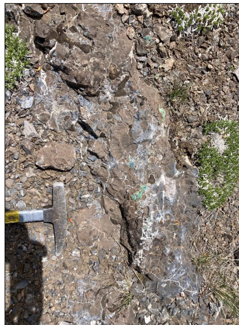
Eliza Follow-up Sampling 2022 Dolomite micro-breccia, showing calcite filling and copper mineralization
