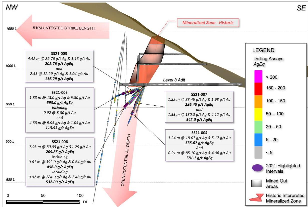
**Figure 1: Long section showing mined out stopes and highlighted intercepts**
